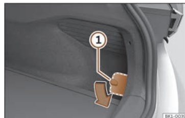
Fig. 51 On the lower right-hand side of the luggage compartment trim: cover with cutting lines.
