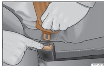
Fig. 20 Release the seat belt's buckle.
