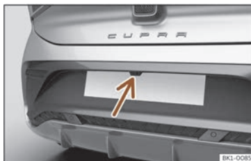
Fig. 100 In the rear bumper: location of the reverse assist camera.
