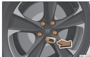
Fig. 165 Wheel: wheel nuts with caps.
