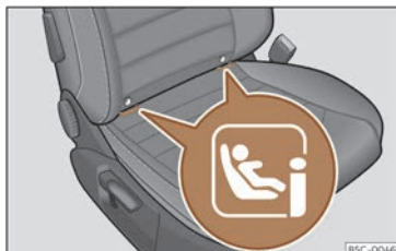
Fig. 36 Front passenger seat: i-Size retaining rings.
