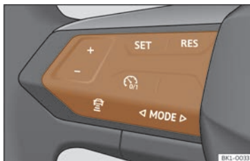
Fig. 101 On the multifunction steering wheel: buttons to operate the speed limiter.
