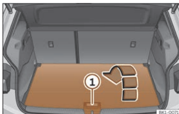
Fig. 137 In the luggage compartment: open the second luggage compartment floor.
