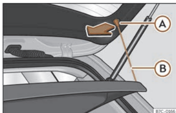
Fig. 134 In the luggage compartment: removing and fitting the shelf.
