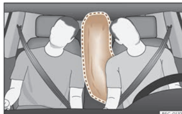
Fig. 28 Fully inflated central airbag (deployment zone).
