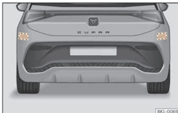
Fig. 98 Rear view of the vehicle: radar sensor zones.
