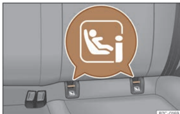
Fig. 35 Rear seat: ISOFIX or i-Size securing rings.
