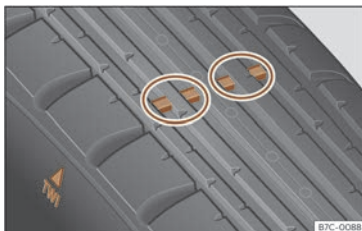
Fig. 162 Tyre profile: tread wear indicators.
