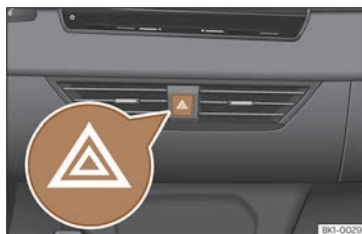
Fig. 40 Dash panel: hazard warning lights switch
