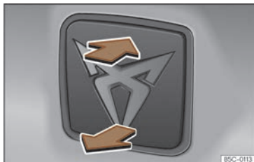
Fig. 67 Rear lid: opening from outside.
