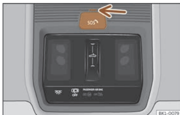
Fig. 41 On the roof console: voice service controls
