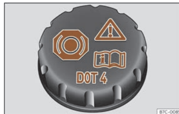
Fig. 159 Front compartment: brake fluid reservoir cap.
