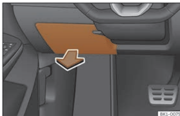
Fig. 151 On the driver's side dashboard: fuse box cover.
