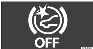
Fig. 109 On the instrument panel display: Front Assist deactivated indication.
