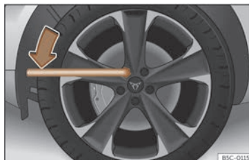
Fig. 167 Wheel change: loosen the wheel nuts.
