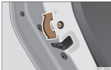
Fig. 66 Childproof lock on the left hand side door.
