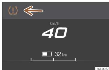
Fig. 164 Instrument panel: warning of loss of tyre pressure.
