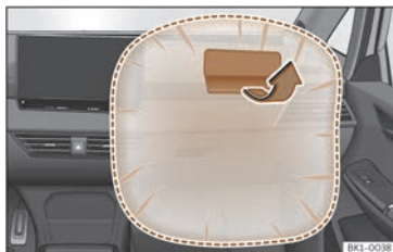
Fig. 24 Front passenger airbag located in dash panel.
