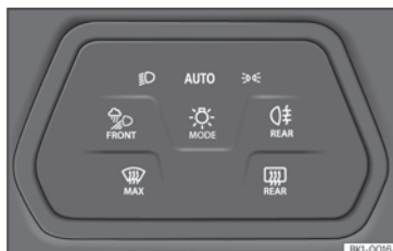
Fig. 81 Dash panel: lights control.
