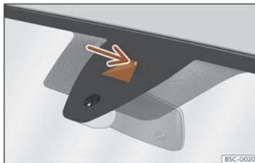
Fig. 97 On the windscreen: field of vision of the Lane Assist system.
