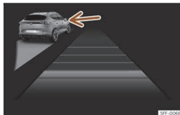
Fig. 104 On the instrument panel display: ACC active, vehicle detected in an outer lane.
