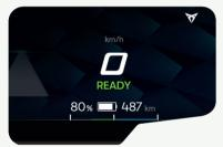
Ready: Vehicle on and stopped, ready to drive The Digital Cockpit displays:
