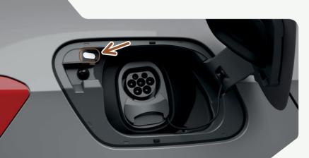
The connector remains locked during the charging process.
