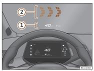
Fig. 5 In the driver's field of view: Proximity HUD (1) and AR HUD (2).
