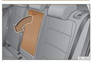
Fig. 79 Folding rear centre armrest (schematic view).
