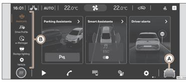
**Fig. 12** Schematic representation: Assist systems and vehicle settings
