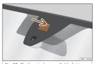
**Fig. 97** On the windscreen: field of vision of the Lane Assist system.
