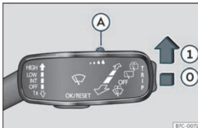
Fig. 97 Wiper lever: adjust the rain sensor (A)
