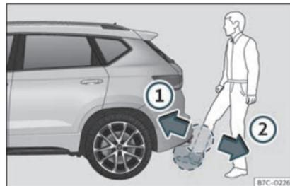
Fig. 85 Rear lid with sensor-controlled opening (Easy Open).
