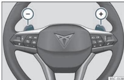
**Fig. 144** Steering wheel: automatic transmission levers
