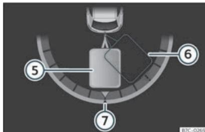
**Fig. 189** Instrument panel display: engage reverse gear
