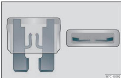
Fig. 48 Image of a blown fuse.
