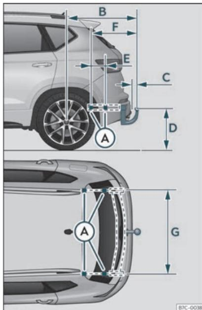
**Fig. 196** Limits and attachment points for retrofitting a towing bracket.
