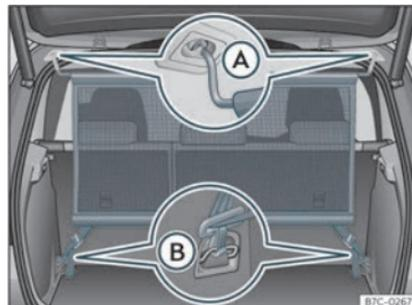
**Fig. 122** Net partition fitted.
