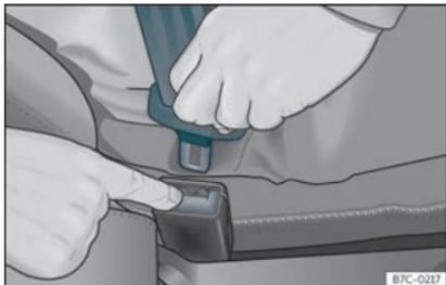
**Fig. 10** Release the seat belt's buckle.
