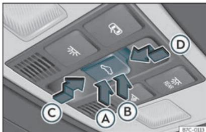
Fig. 89 On the interior roof lining: sunroof button.
