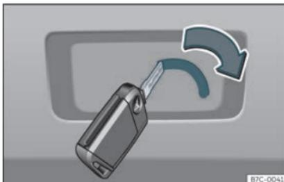
**Fig. 87** Detail of the luggage compartment: emergency unlocking
