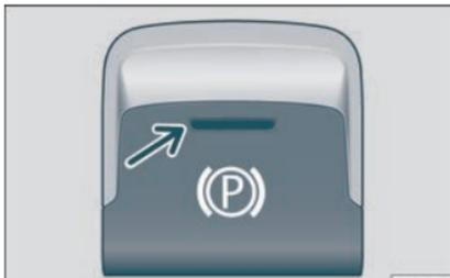
**Fig. 175** In the lower part of the centre console: electronic parking brake button
