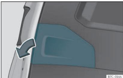
**Fig. 51** Rear lid open: remove the cover.
