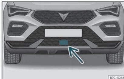
Fig. 148 On the front bumper: radar sensors.
