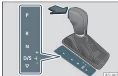
**Fig. 142** Selector lever lock.
