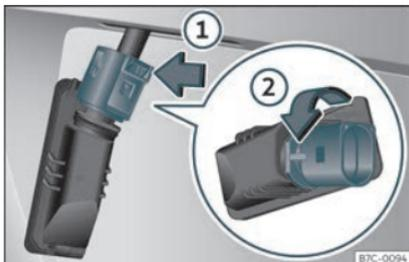
**Fig. 54** number plate light: remove the bulb holder.
