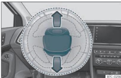
Fig. 13 Driver airbag located in steering wheel.
