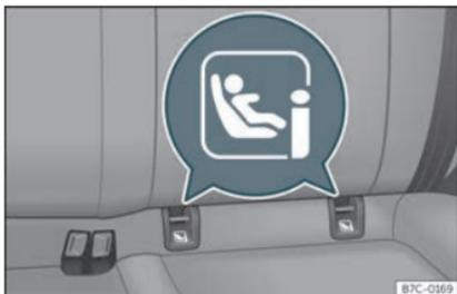
**Fig. 25** Rear seat: ISOFIX/i-Size securing rings.
