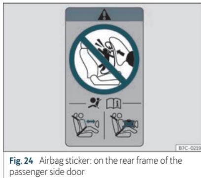
Fig. 24 Airbag sticker: on the rear frame of the passenger side door
