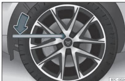
Fig. 34 Wheel change: loosen the wheel nuts.
