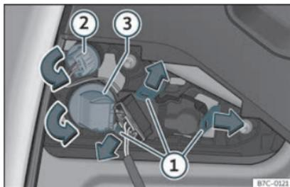
**Fig. 52** Remove the bulb holder.
