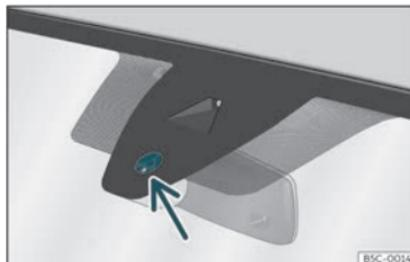
**Fig. 130** Windscreen humidity and temperature sensor.
