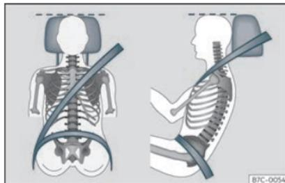
**Fig. 3** Correct belt web and headrest positions
