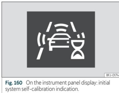
**Fig. 160** On the instrument panel display: initial system self-calibration indication.
