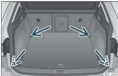
**Fig. 116** In the luggage compartment: fastening rings.
