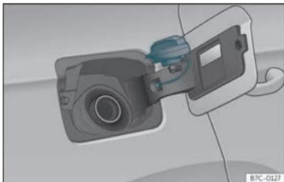
**Fig. 197** Fuel tank flap with tank cap attached.
