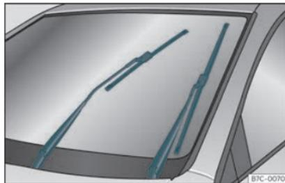
Fig. 37 Wipers in service position.
