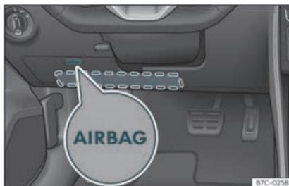
**Fig. 17** On the driver side: location of the knee airbag
