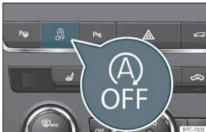
**Fig. 141** Centre console: Start-stop system button.
