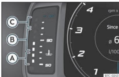
Fig. 61 Engine coolant temperature indicator.
