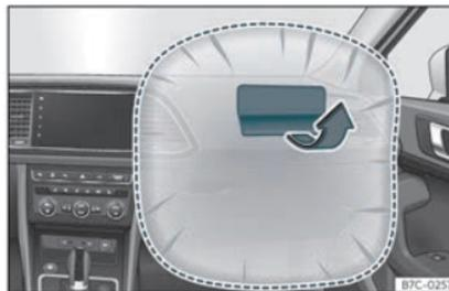
Fig. 14 Front passenger airbag located in dash panel.
