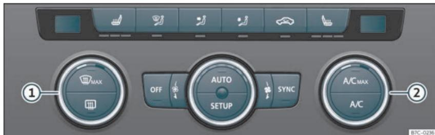
Fig. 129 In the centre console: Climatronic controls.
