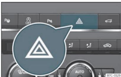
Fig. 95 Dash panel: hazard warning lights switch
