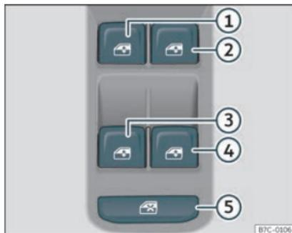
**Fig. 88** Detail of the driver's door: window controls.
