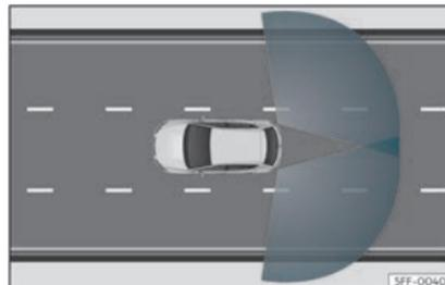
Fig. 152 Sensor detection zones
