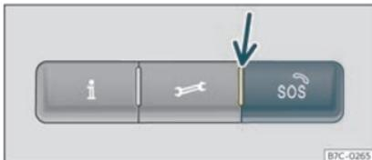
**Fig. 29** On the roof console: voice service controls
