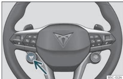
**Fig. 147** Multifunction steering wheel\*: button to change the driving profile.
