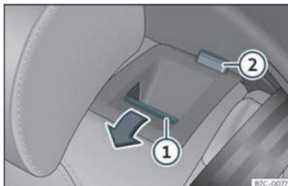
**Fig. 107** Rear seat: folding the backrest.
