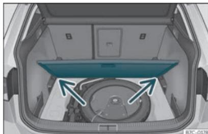
**Fig. 115** Variable luggage compartment floor: inclined position.
