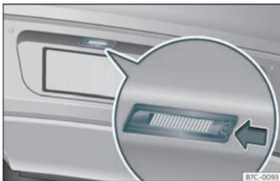
**Fig. 53** In the rear bumper: Number plate light.
