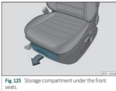
**Fig. 125** Storage compartment under the front seats.
