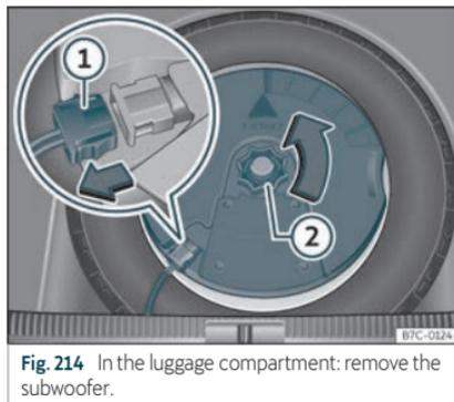
**Fig. 214** In the luggage compartment: remove the subwoofer.
