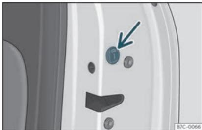
**Fig. 80** Locking the door manually.
