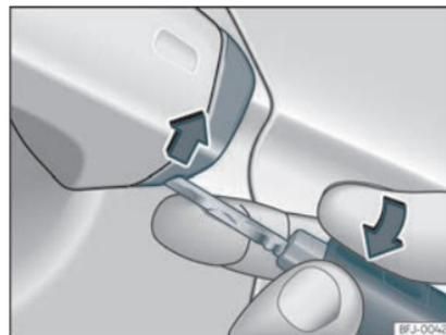
**Fig. 79** Driver door handle: lever the cover off
