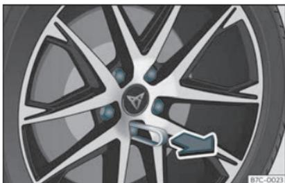
Fig. 32 Wheel: wheel nuts with caps.
