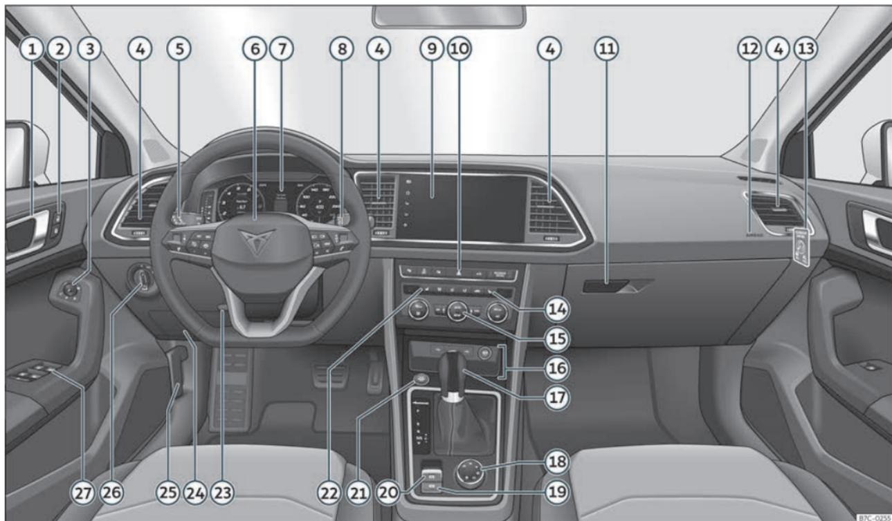
Fig. 56 Instruments and controls.
