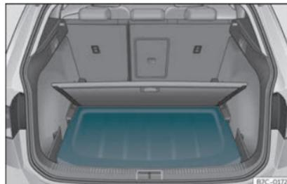
Fig. 113 In the luggage compartment: fitting the rear shelf.
