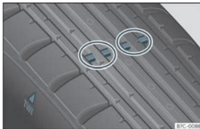
Fig. 210 Tyre profile: tread wear indicators.
