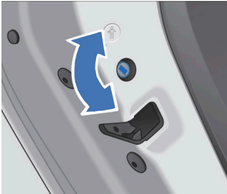
Deactivate the childproof lock mechanically using the key.
