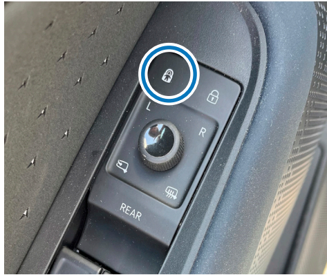
Deactivate the childproof lock electronically in the door trim.
