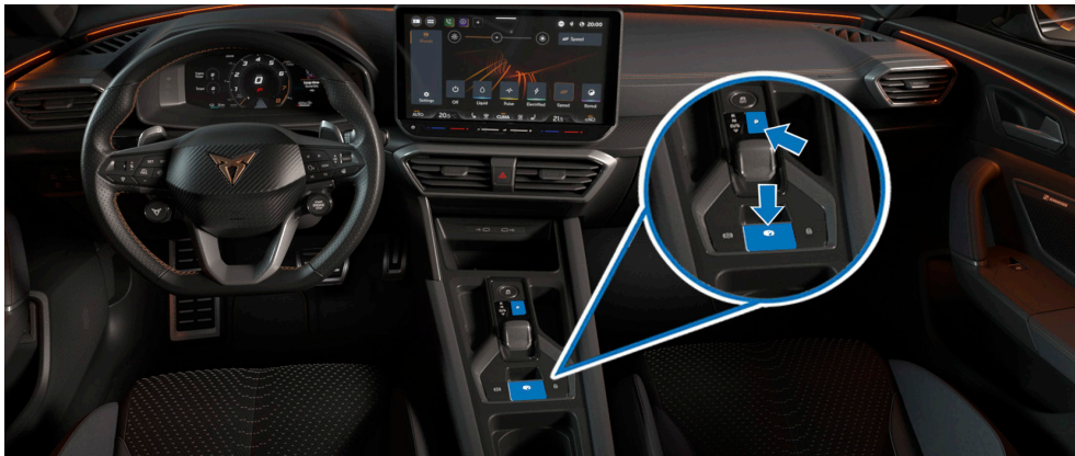
Vehicles with automatic gearbox without selector lever: press P button and activate the electric handbrake.
