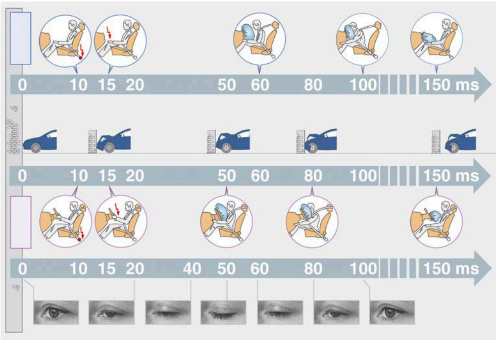
The safety systems are deployed depending on the type of accident or direction of impact (ms = milliseconds).
