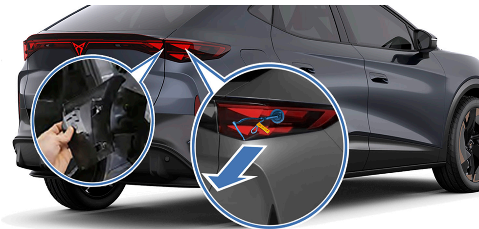
Cut-out connection in the rear of the vehicle behind the right tail light cluster (Example TAVASCAN)
