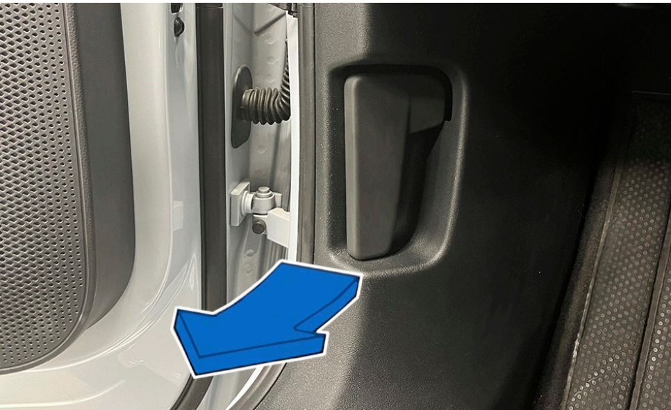
In the footwell on the driver's side: release lever for the bonnet.
