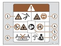
**Fig. 64** High-voltage battery warning lettering.
