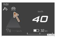
Fig. 25 Eco-efficient driving assistance indication (schematic representation).
