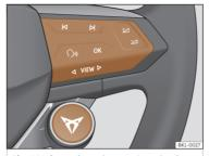
Fig. 93 Controls on the steering wheel.
