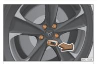
Fig. 198 Wheel: wheel bolts with caps.
