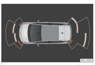
Fig. 143 Parking aid view on the Infotainment system display.
