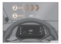
Fig. 22 In the driver's field of view: Proximity HUD (1) and AR HUD (2).
