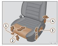
**Fig. 95** Front seats: manual seat adjustment.
