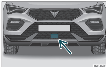
Fig. 148 On the front bumper: radar sensors.
