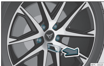
Fig. 32 Wheel: wheel nuts with caps.
