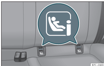
Fig. 25 Rear seat: ISOFIX/i-Size securing rings.
