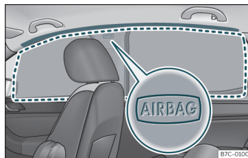
Fig. 21 Location of head-protection airbags.
