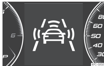
Fig. 158 On the instrument panel display: advance warning indications.
