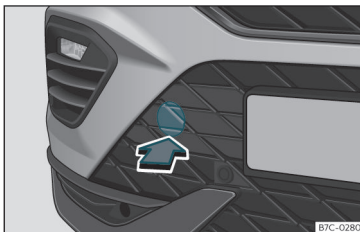
Fig. 41 On the right side of the front bumper: remove the cover.
