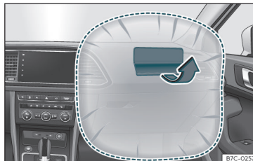
Fig. 14 Front passenger airbag located in dash panel.
